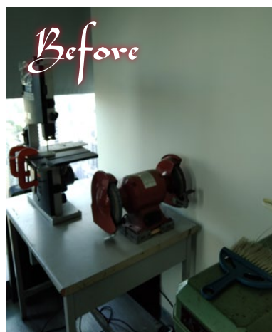
Before improvement: No warnings were posted on the grinder, and no goggles were worn during the operation
